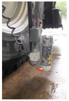
Both of the units are outfitted with strong magnets so that they can be placed on any magnetic surface without screws. The unit is simply placed and then plugged in to a 12v or 24v output (the unit is delivered for 12v or 24v).
